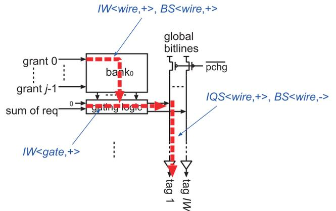
Fig. 24 Parameters that impact the delay in the tag RAM.
