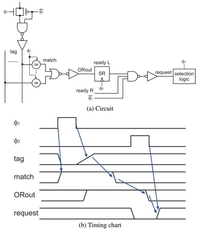
Fig. 17 Circuit from tag drive to selection logic.
