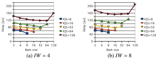
Fig. 22 Tag RAM delay for various bank sizes.
