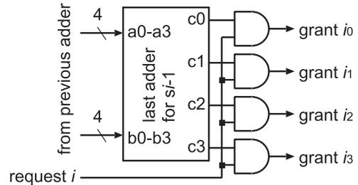
Fig. 6 Grant output circuit with  $IW = 4$ .
