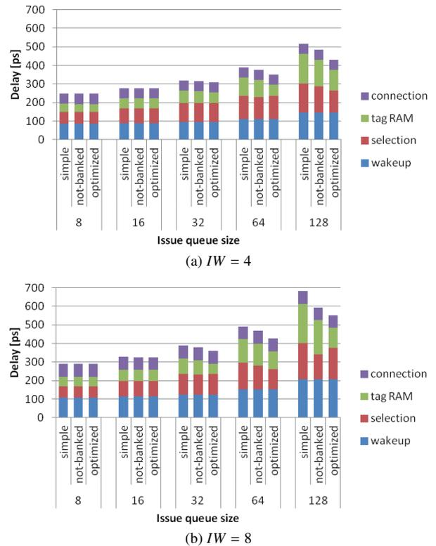
**Fig. 27** Total delay of issue queue with design optimizations.
