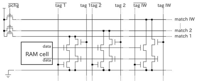
Fig. 4 CAM cell circuit for tag comparison.
