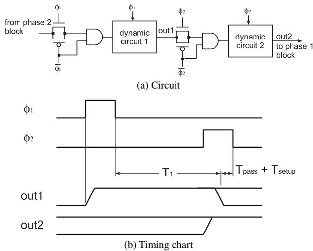
Fig. 15 Two-phase dynamic circuit.
