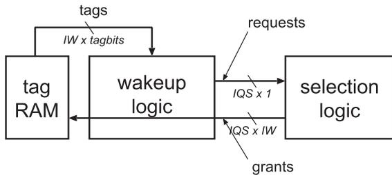
**Fig. 11** Layout of wakeup logic, selection logic, and tag RAM.
