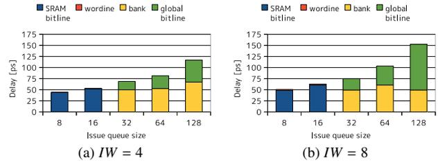
Fig. 23 Delay of tag RAM with optimal bank configuration.
