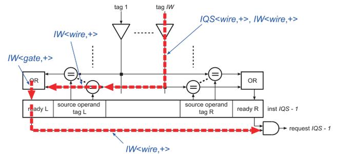
Fig. 19 Parameters that impact delays in the wakeup logic.
