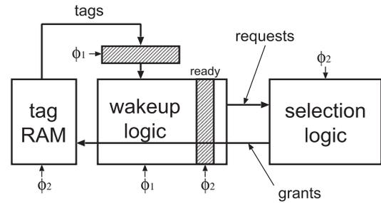
Fig. 16 Insertion of clocks and latches.
