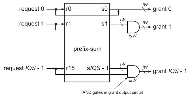
Fig. 8 Top-level diagram of selection logic.
