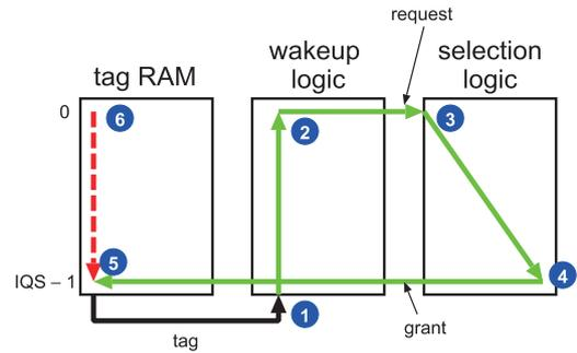
**Fig. 12** Path simply connecting the critical path of each component.
