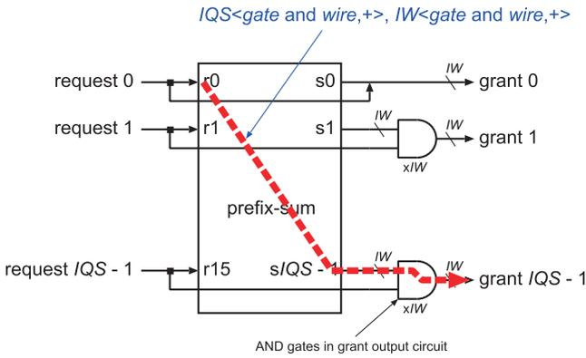
Fig. 21 Parameters that impact the delay in the selection logic.
