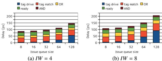
Fig. 18 Delay of wakeup logic.
