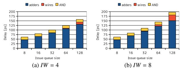
Fig. 20 Delay of selection logic.
