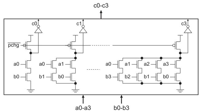
Fig. 7 Adder for selection logic ( $IW = 4$ ).
